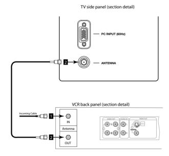
Figure 4. Connecting the VCR with antennas or wall outlet cable.
